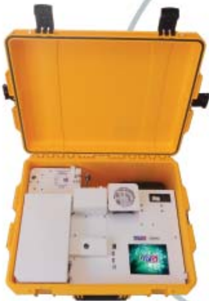
Companion 2 Portable GC (with Purge & Trap Concentrator)
