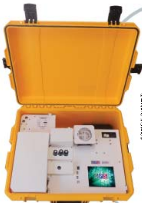
Companion 2 Portable GC With Dynamic Headspace Concentrator, (Vial Heater, "Cathedral" Trap, Sample Valve)
