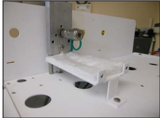
Detector Body Reactor Cell Collector
