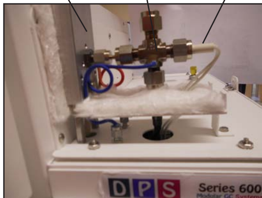
Detector Block Detector Body Igniter
