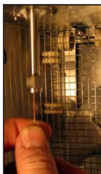
Place Column into Injector
