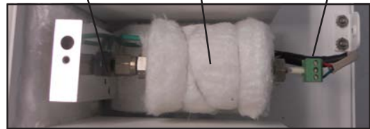
Detector Body Reactor Cell Collector
